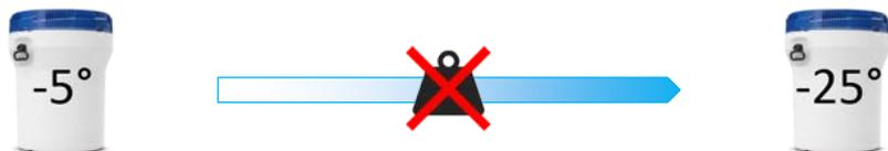
**Attention!** The volume of drums filled with water-based contents can increase by 10%. The chances that drums will distort are real and it will reduce the stability of a drum stack on a pallet. Please maintain a maximum filling level of 90% and test the stability of a pallet stacking.
