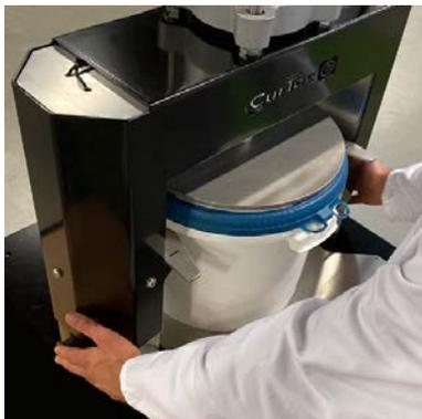
3. Press both red buttons at the same time. The rubber stamp will press down the lid until it snaps onto the container.
