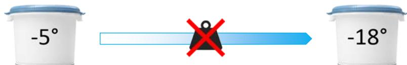
**Attention!** The volume of containers filled with water-based contents can increase by 10%. The chances that containers will distort is real and it will reduce the stability of a container stack on a pallet. Please maintain a maximum filling level of 90% and test the stability of a pallet stacking.
