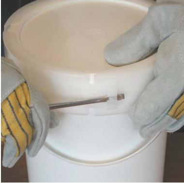
1. Break the buckle on the clamp by using a screw-driver. Insert the screw-driver into the buckle from your right-hand side.
