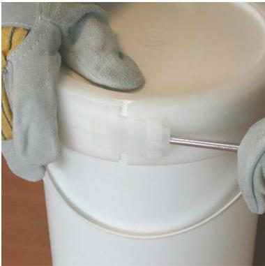
2. Insert your screw-driver from your left-hand side and lift the right clamp-end from the buckle.
