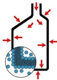
it comes to plastic packaging, escape results in product loss, contamination and damage. CurTec has found a solution for permeation of chemicals through plastic: fluorination.
