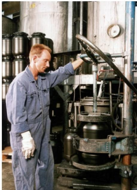
Colloidal dispersions are formed by dissolving graphite powder in water or oil and serve as a lubricant for forging steel and a release agent in injection moulding of aluminium and zinc. The dispersions, after a certain amount of time, must be rolled in order to mix the ingredients. Panelling (where the drums sides go concave) can also occur during the often long road to the consumer.
